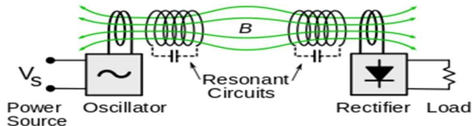
Diagram of the resonant inductive wireless power system demonstrated by Marin Soljačić's MIT team in 2007. The resonant circuits were coils of copper wire which resonated with their internal capacitance (dotted capacitors) at 10 MHz. Power was coupled into the transmitter resonator, and out of the receiver resonator into the rectifier, by small coils which also served for impedance matching
