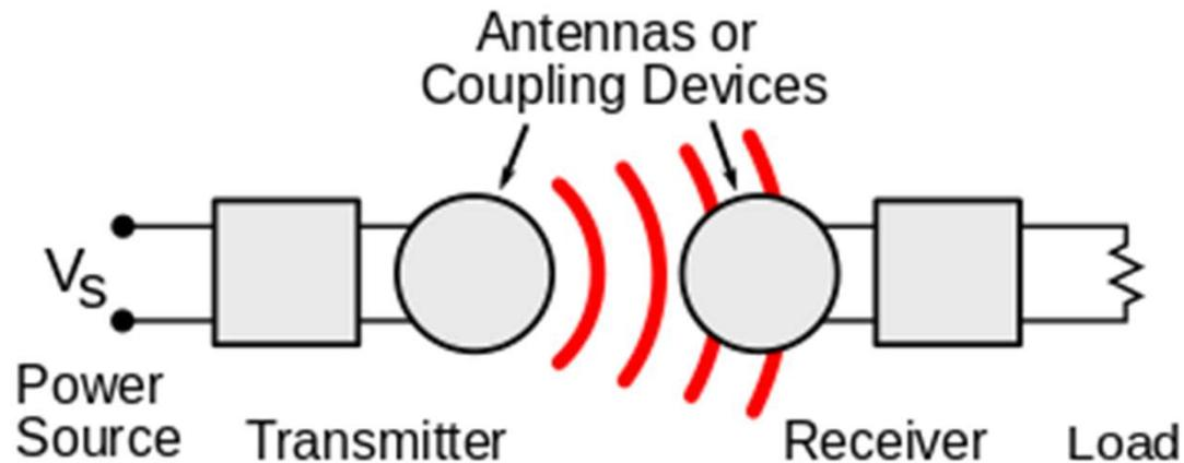
In general a wireless power system consists of a "transmitter" connected to a source of power such as mains power line, which converts the power to a time-varying electromagnetic field, and one or more "receiver" devices which receive the power and convert it back to DC or AC electric current which is used by an electrical.
