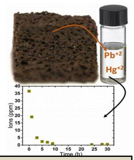
99% of Lead & Mercury ions removed from waste water over 30 hours
