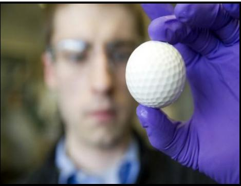
**Spent Coffee-Bioelastomeric Composite Foams** used for the removal of Pb<sup>2+</sup> and Hg<sup>2+</sup> from Water
