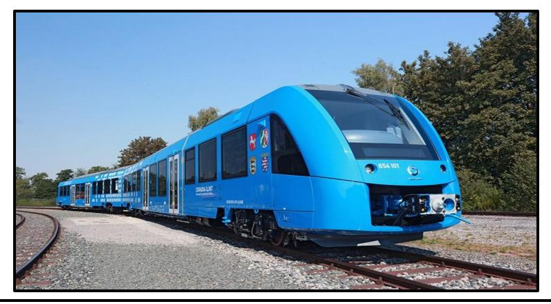
The hydrogen, aka "hydrail," train is powered by a hydrogen fuel cell and emits nothing but steam and condensed water-with Speeds up to 87 mph & storage capacity for a 497 mile range
